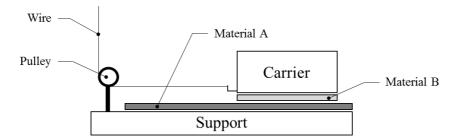
Figure 1: Schematic of the frictional test setup presented in DIN 14882 (adapted from [2])
