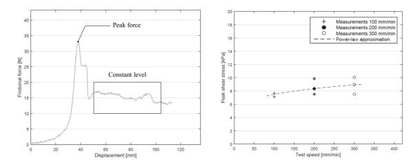
Figure 2: (Left) Typical force vs displacement test result; (Right) Evolution of peak shear stresses with respect to test speeds for  $0^{\circ}/0^{\circ}$  inter-ply slip experiments
