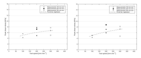
Figure 3: Evolution of peak shear stresses with respect to test speeds for inter-ply slip experiments (left) 0°/90° (right) 90°/90°
